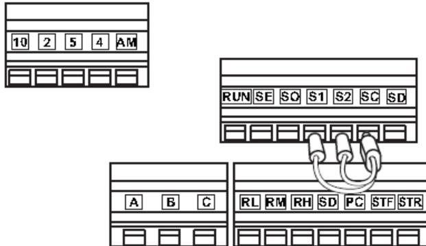
The input signals are set to sink logic (SINK) when shipped from the factory.
