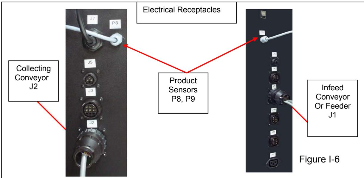
8. Plug the collecting conveyor cable into the J2 receptacle located on the LH side panel of the FIT 36 electrical enclosure. See figure I-6.
