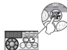
Operation 2: ..... Switch OFF the power once, then switch it ON again after the indicator of the operation panel turns OFF.
