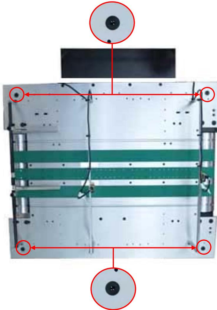
Remove 2 flat head screws from the corners on the Operator's side
